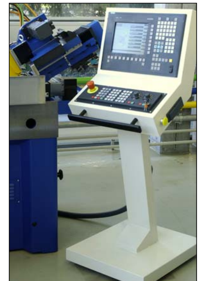
Siemens 840 D control unit
