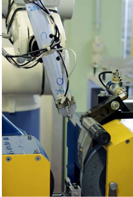
2 Using an existing interface, a robot from an external supplier was simply integrated into the automation concept
