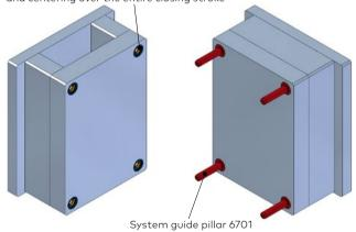
The tool concept can be significantly simplified with the Agathon Guiding System Plus:
