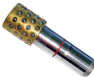
Wear image on an Agathon Mini Fine Centering unit after 3.6 million cycles
